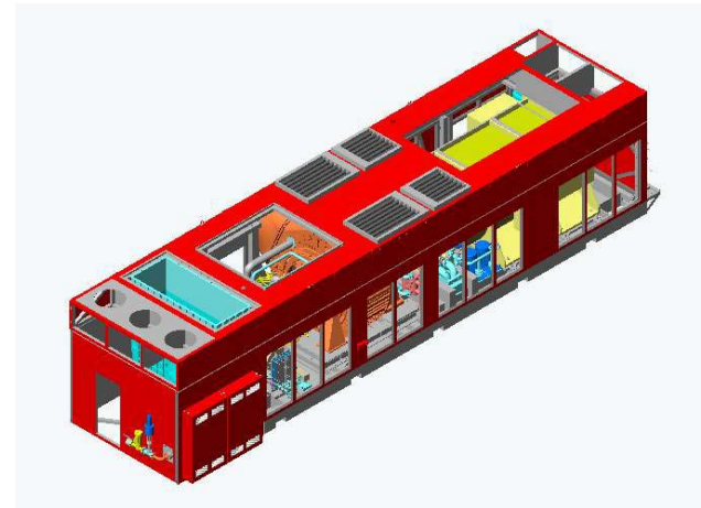
Turbomach's gas turbine plant model RB211
